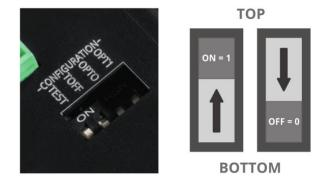
DIP switches interface for simple and fast configuration
